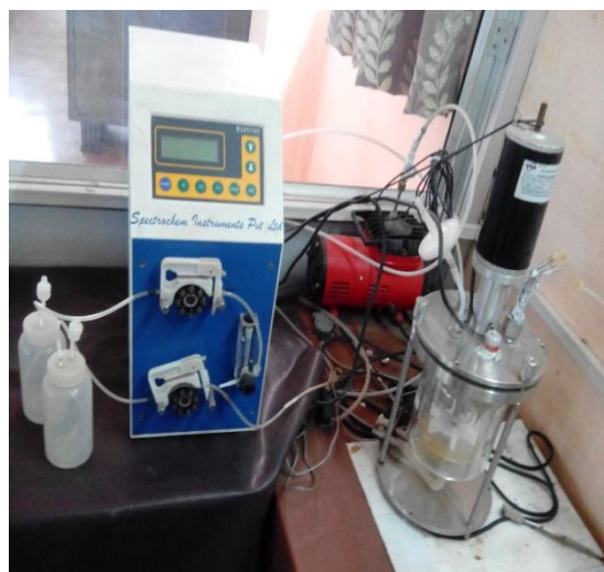
Fig 2 Biotron 1 Liter Bioreactor showing reactor with motor connected to processor unit and compressor
