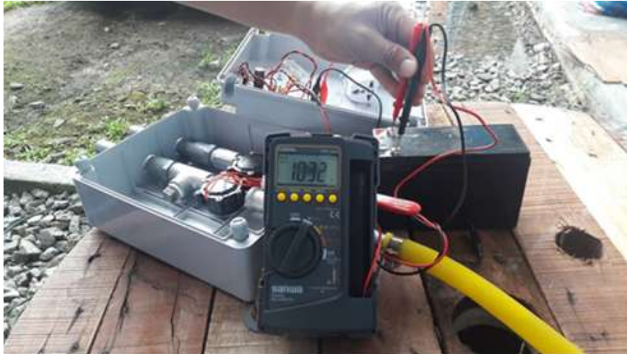
Fig. 9:- Battery voltage before charging without using current booster.
