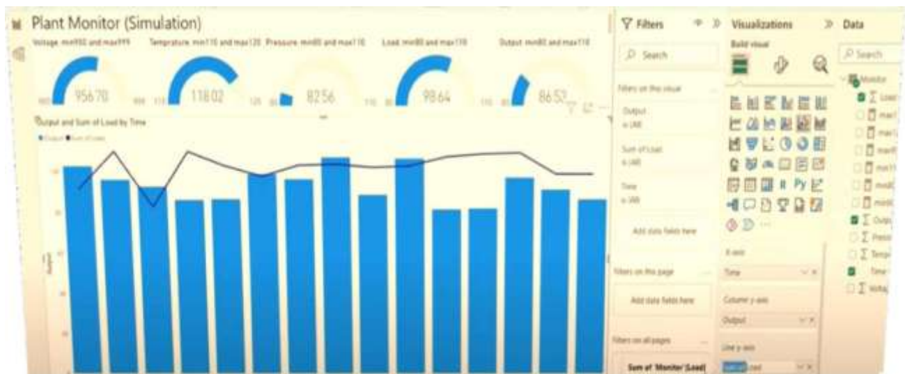
Fig 3.2:- Grid Utility modelled using Power BI to analyse the load profile of the generating station for a virtual timeseries data set.
