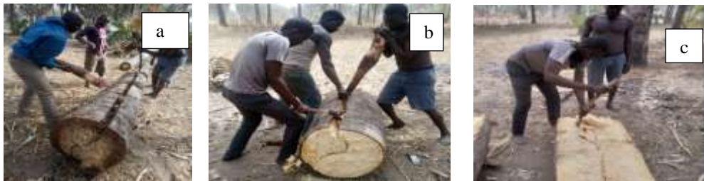
Photo 1:- Borassus wood splitting technique.
