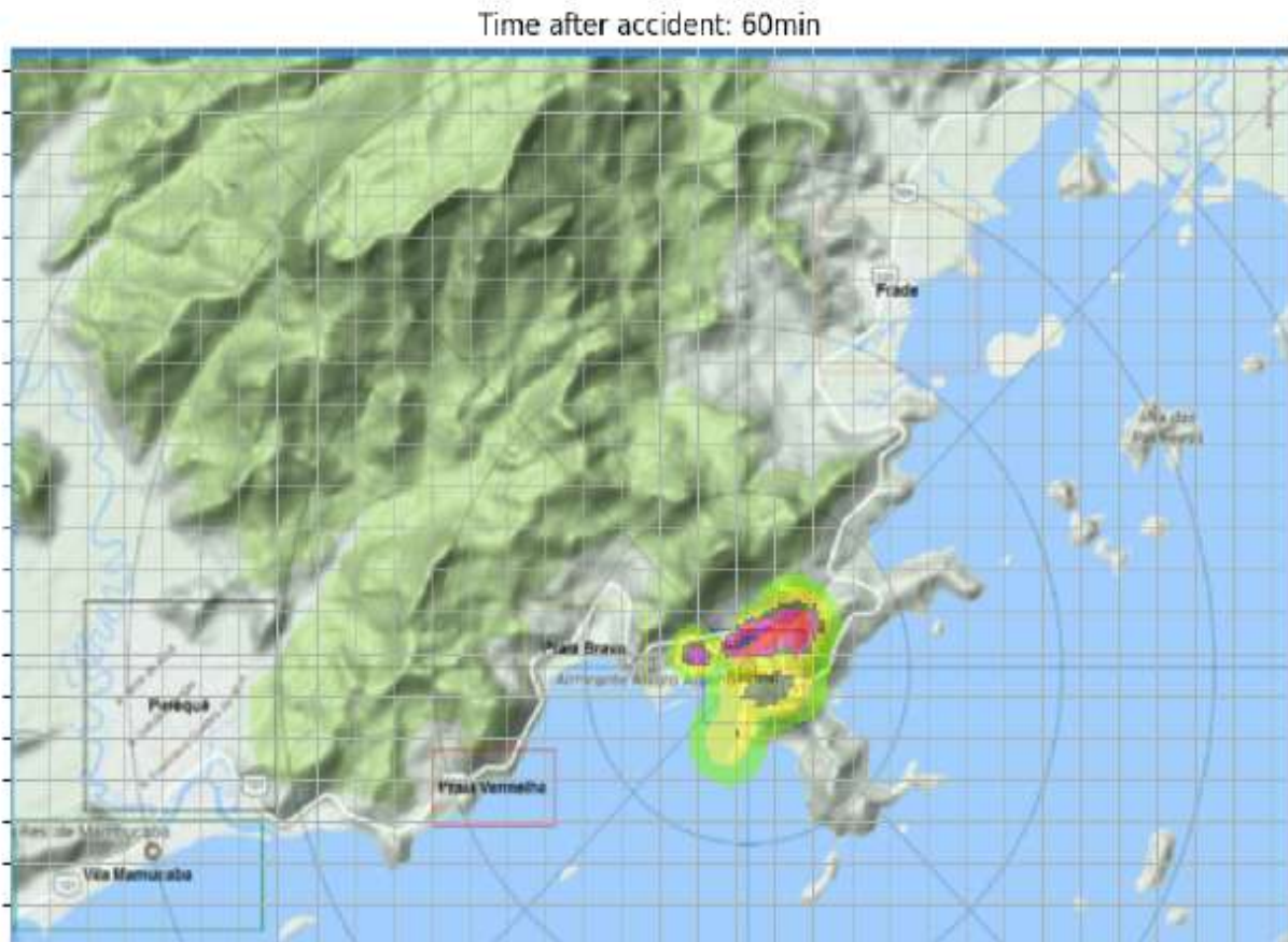
Figure 5: Dose rate distribution map for cycle 4 of the hypothetical accident. Source: from authors in 2023.
