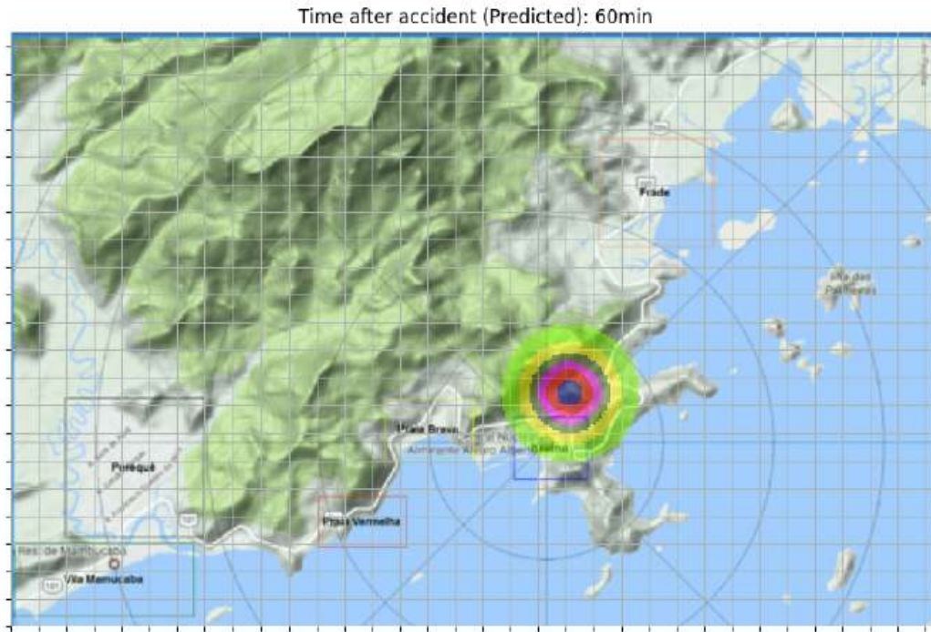
Figure 10:- Dose rate distribution map estimated by the model for cycle 4 of the hypothetical accident. The colors represent the doses on the scale of Figure 8.
