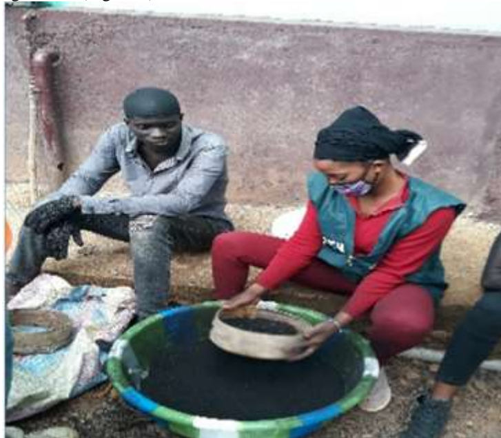
Figure 7:- Sieving the powder of the herbaceous charcoal obtained.
