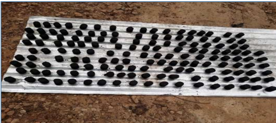
Figure 10:- Briquettes final drying.
