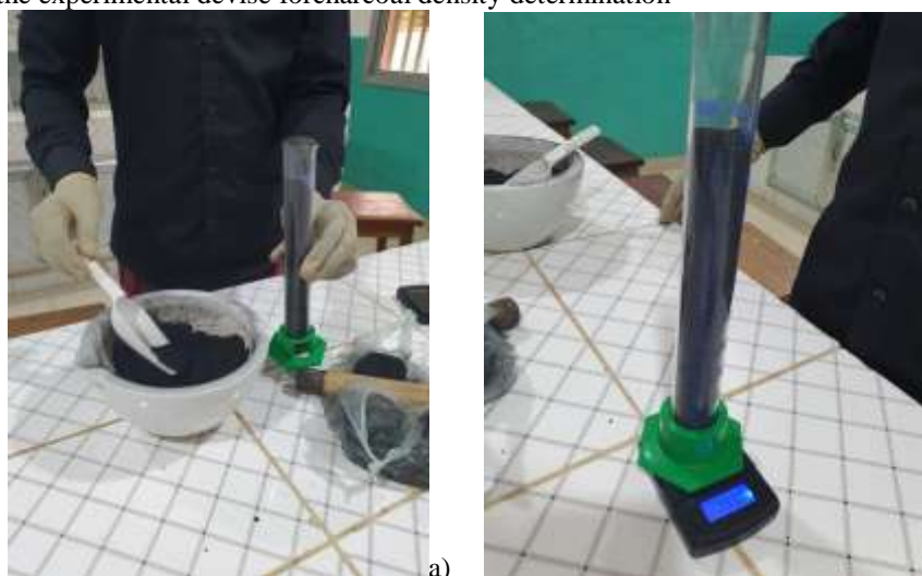
Figure 11; -Charcoal density determination a) filling the graduated cylinder, b)weighing graduated cylinder filled with ecological charcoal powder.
