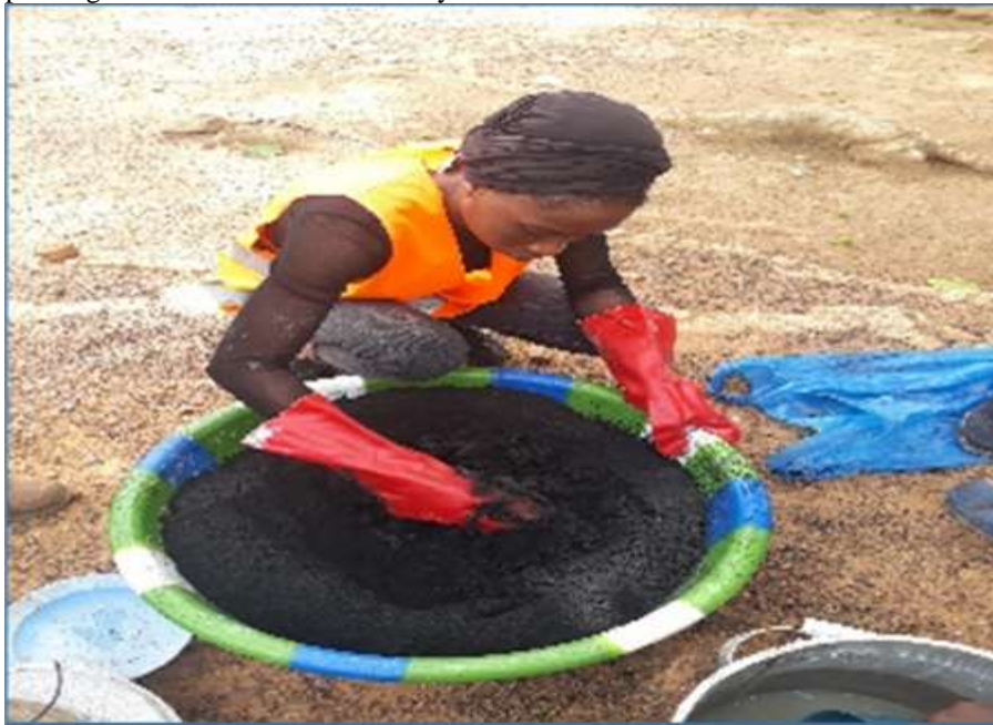
Figure 8:- Sieving the powder of the herbaceous obtained.
