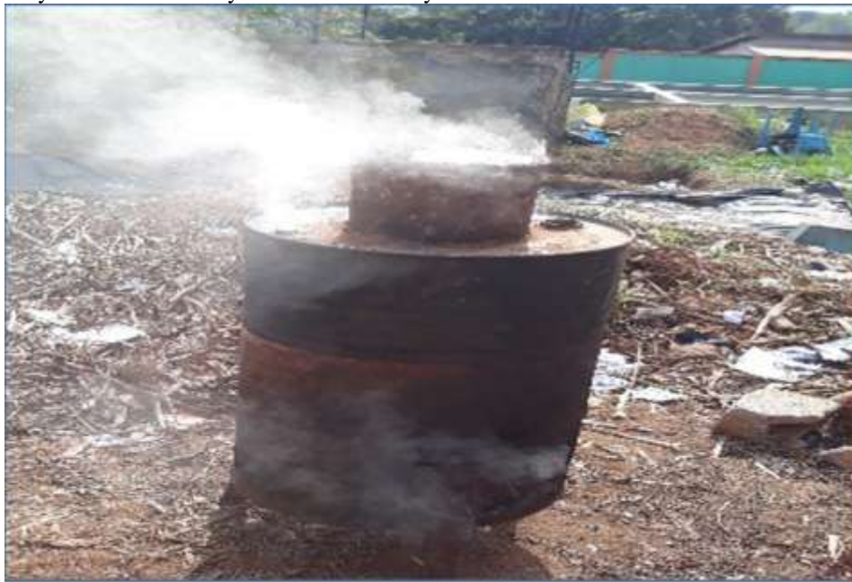
Figure 5:- Carbonization of the herbaceous in the oven.
