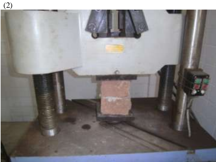
Photo 1:- Bending strength test (three points) on CEB.
