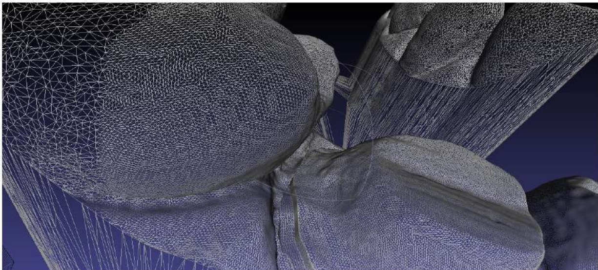
Fig.1:- Illustration of the polygon meshes formed during the digital 3D object reconstruction process.
