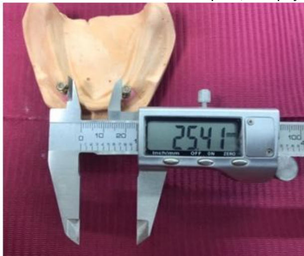
Fig (4):- Distance between implant analogs measured by the electronic digital caliper.
