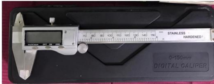
Fig (3):- The electronic digital caliper.
