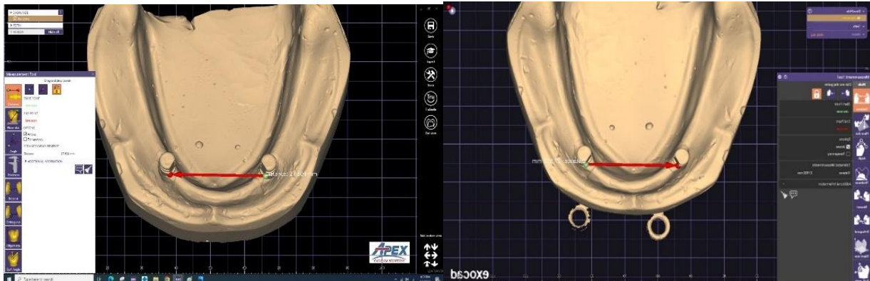
Fig (6 a & b):- Distance between the two implant analogs measured from the same reference pints by Software’s of DofFreedom X5 premium and Medit T300-T500 dental lab scanners.
