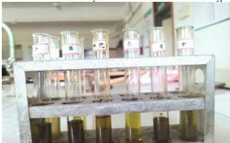
Figure 1. and Table 2. shows the solubility test of leaves extract from different type of Solvent
