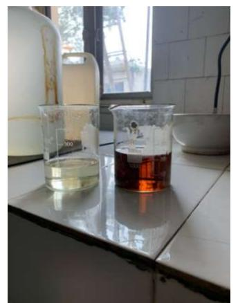
Fig.2:- Visual Comparison of waste and lab recovered Sulphuric acid.
