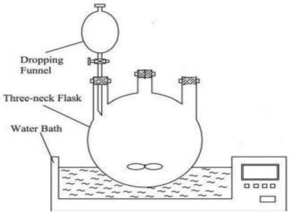
Fig. 1:- Setup for waste Sulphuric Acid Oxidation process.
