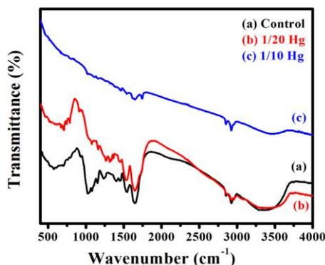
**Fig.1** FTIR spectra of control and mercury exposed *C. mrigala* Liver (a) control, (b) 1/20<sup>th</sup> HgCl<sub>2</sub>, (c) 1/10<sup>th</sup> HgCl<sub>2</sub>
