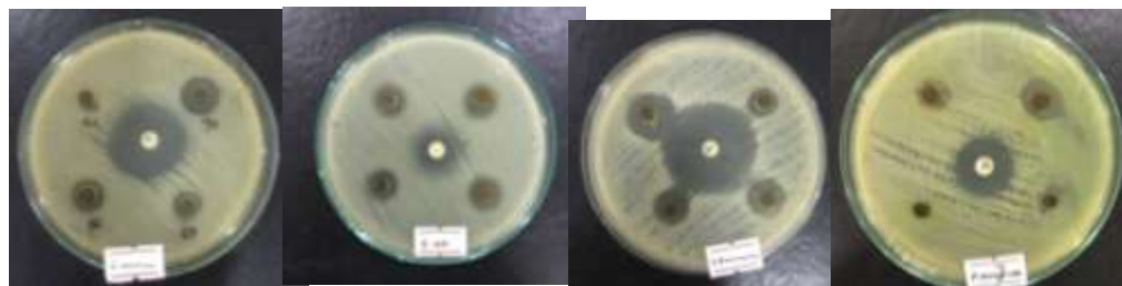
Antibacterial activity of neem-mediated AgNPs at temperature variation against bacterial pathogens: S. aureus , E. coli , K. pneumoniae , P. aeruginosa respectively
