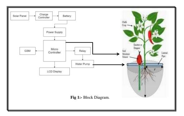
When the power supply is given to ATmega 328p microcontroller, the moisture sensors transmit data to the microcontroller then monitors the data and finally send to the receiving section where the user's smartphone receives data and accordingly show the data of soil moisture level.
