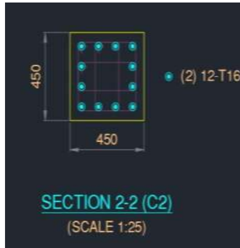
Fig 6.7:- Column Reinforcement Detailing.
