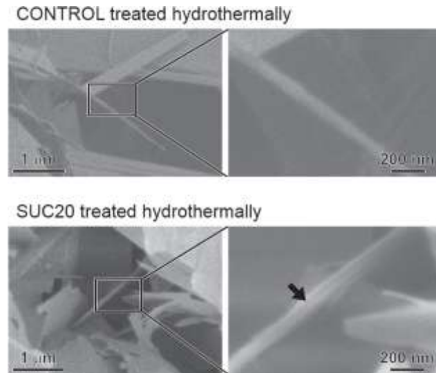
Figure 3:- SEM magnification images of Control or Calphos and suc-20 under hydrothermally treatment (at 180°C for 3 hours), with an arrow which indicate a dark line at center of HAP nanocrystal system.
