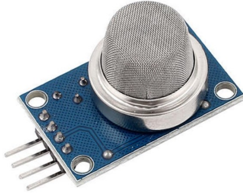
Fig 8:- Gas and Smoke Sensor.
