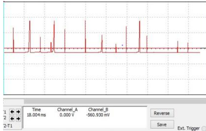
Fig.9. (b).Output of PLL resonator signal conditioning unit
