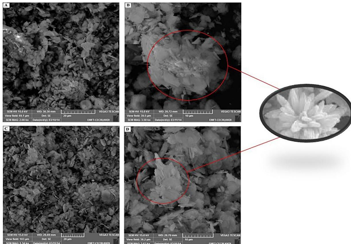
**Fig. 4.** Shows SEM image of CuO nanoparticles synthesized with two different concentrations of NaOH at (a & b) 0.3M and (c & d) 0.5M
