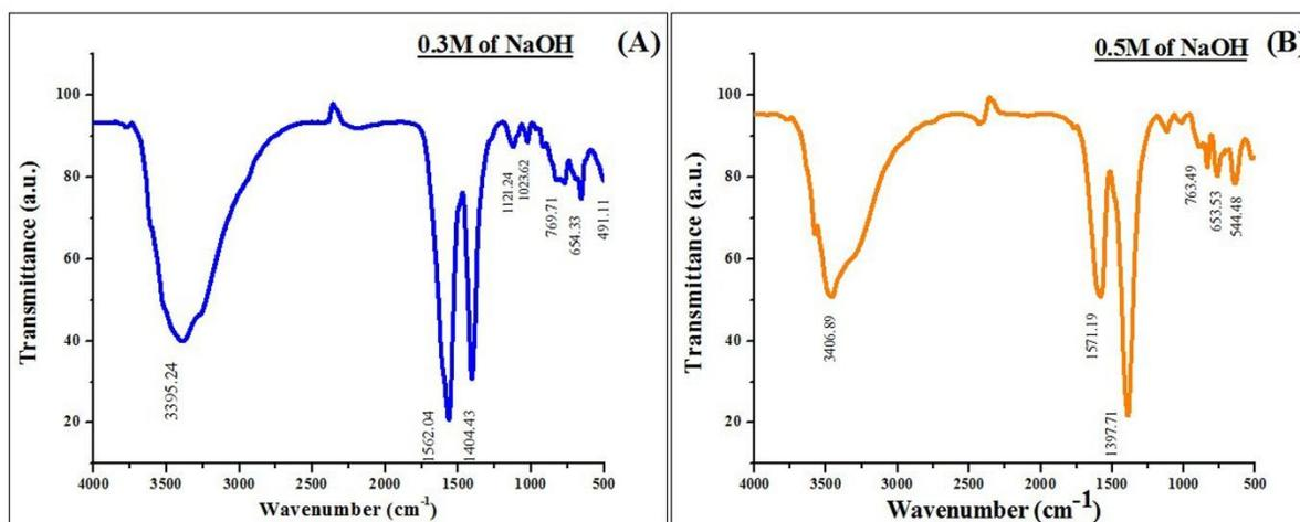
**Fig. 2.** FTIR spectra of CuO nanoparticles synthesized at two different concentrations of NaOH at (a) 0.3M and (b) 0.5M
