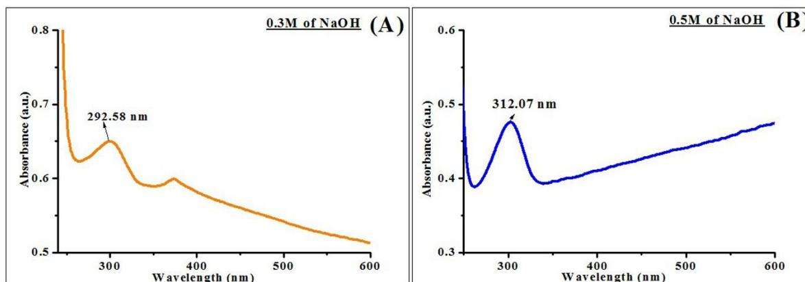
**Fig. 1.** Shows the absorption spectra of CuO nanoparticles synthesized at two different concentrations of NaOH at (a) 0.3M and (b) 0.5M
