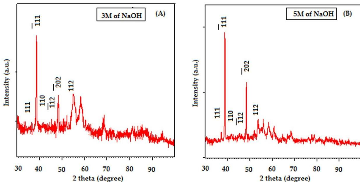
**Fig. 3.** Shows XRD spectra of CuO nanoparticles synthesized with two different concentrations of NaOH at (a) 0.3M and (b) 0.5M.
