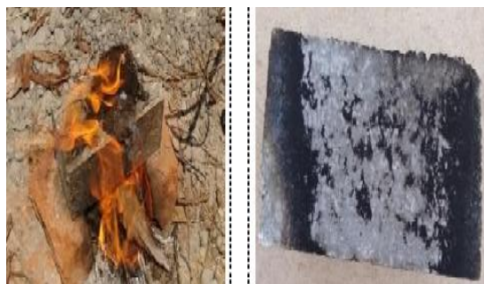
Figure7:-Papercrete Bricks during and after fire test [11]
