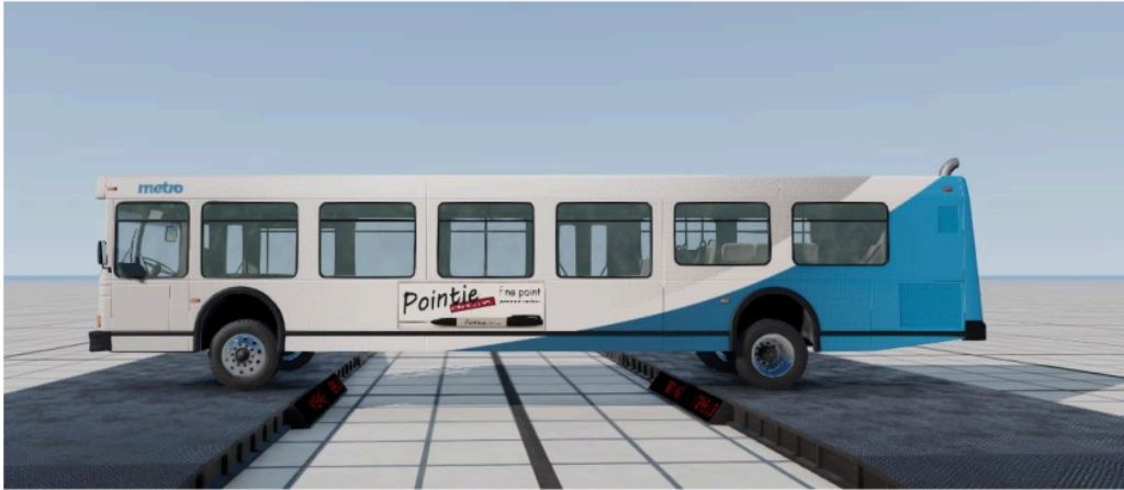
Figure 1.2a: The image of the left side of the bus with the weighing scales.
